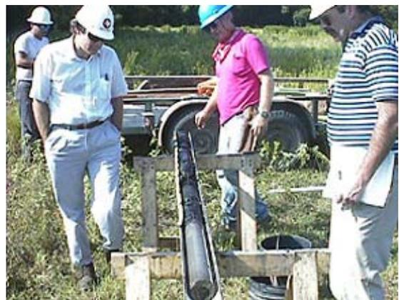
**Figure 3: Core sample from a well (USGS)**
